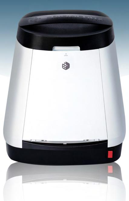
The **Dux**Geldoc specially designed allows high definition images of electrophoresis gel to acquire for documentation. The low-cost Raspberry camera ver 2.0 is adopted to capture high quality gel images. The compact and convenient device take little space. The darkroom is designed to produce high resolution image. Enjoy the high definition gel image using the **Dux**Geldoc.
