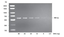
**EZ-Vision® In-Gel Sensitivity** DNA (2.5 ng - 80 ng) was mixed with 6X Agarose Gel Loading Buffer and applied to a 1% TAE agarose gel. Samples were resolved for 1 hour at 6.4 V/cm in 1X TAE buffer. Fluorescent visualization of DNA was achieved with a 500 msec UV exposure using a Sybr Green filter with the Syngene GBox-HR Gel Doc System.
