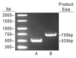
Efficient Amplification of Purified DNA with Extender™ PCR-to-Gel Master Mix. Single copy targets were amplified from 50 ng of pUC19 plasmid (A) or S. aureus genomic DNA (B) for 35 cycles. 10µl of each PCR reaction was directly loaded onto a 1% agarose gel and visualized with a Syngene HR gel doc system.
